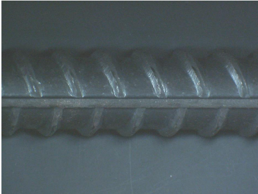
Figure 1 – Example of 'herring bone' rib pattern on bar specimens
