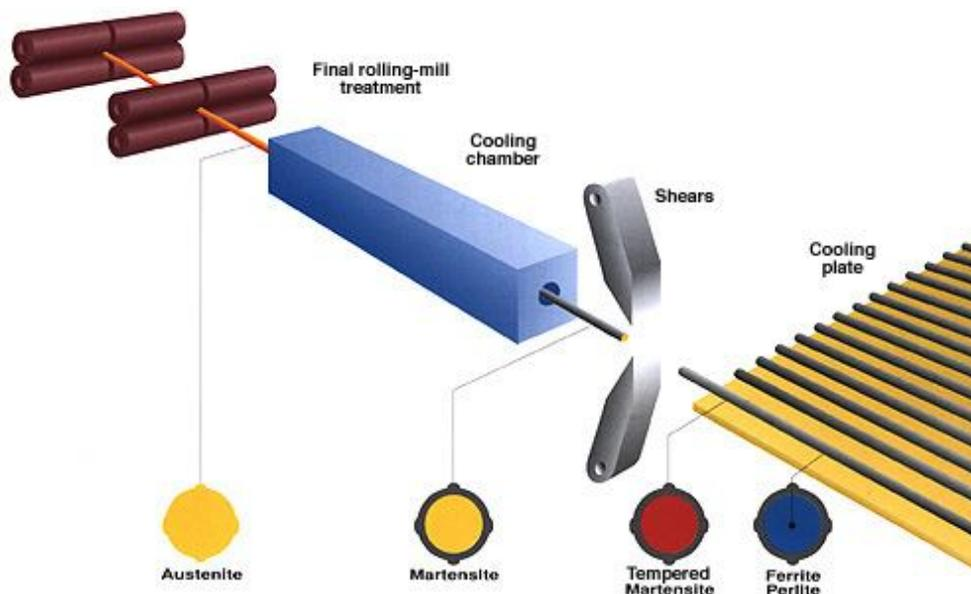
The above schematic diagram illustrates the **Quench & Temper** process which converts low carbon steel into 500 MPa high strength bars with a guaranteed yield strength of 500 MPa.
