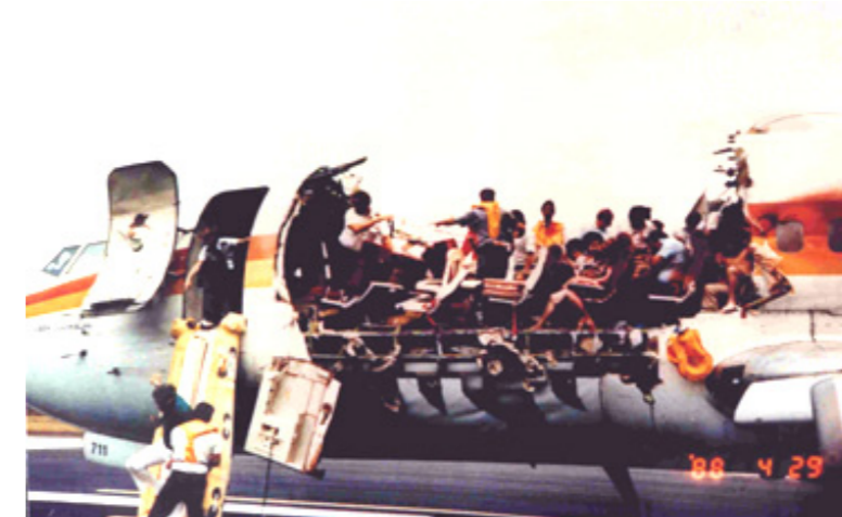
Fig. 14 Aircraft after landing in the Aloha airlines incident. After 89,090 flight cycles on a 737-200, metal fatigue lets the top go in flight.
