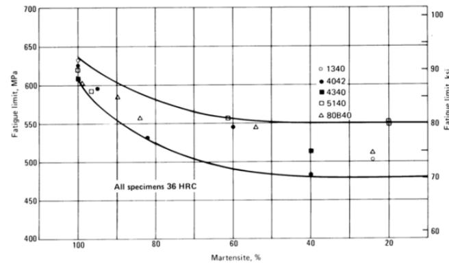
Fig. 4 Effect of martensite content on fatigue limit.
