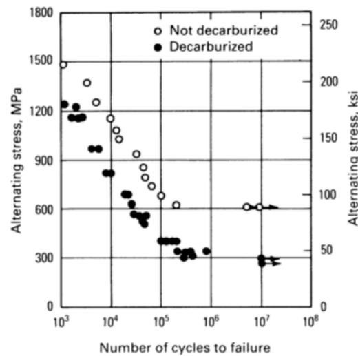
Fig. 9 Effect of decarburization on the fatigue behavior of a steel.
