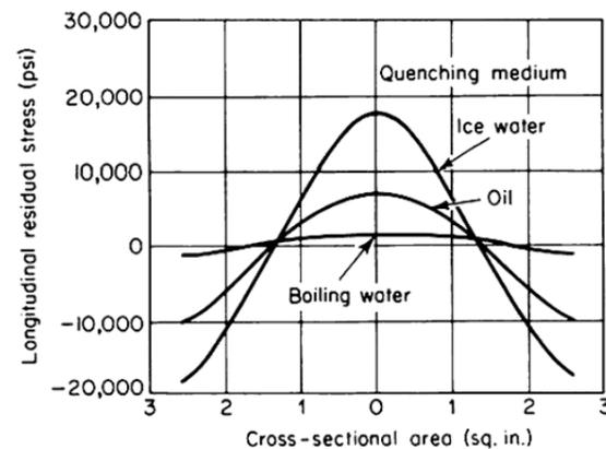
Fig. 13 Residual stress formation along the cross-sectional area for different quenching medium.
