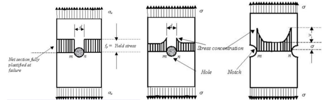
Fig 10 (a) Stress pattern at the point of static failure and (b) stress concentrations in the presence of notches and holes
