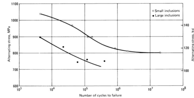
Fig. 11 Effect of nonmetallic inclusion size on fatigue. Steels were two lots of AISI-SAE 4340H; one lot (lower curve) contained abnormally large inclusions; the other lot (upper curve) contained small inclusions.
