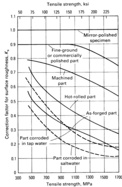
Fig. 8 Surface roughness correction factors for standard rotating-beam fatigue life testing of steel parts.
