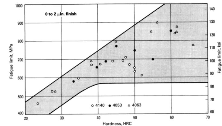
Fig. 3 Effect of carbon content and hardness on fatigue limit of through-hardened and tempered 4140, 4053, and 4063 steels.
