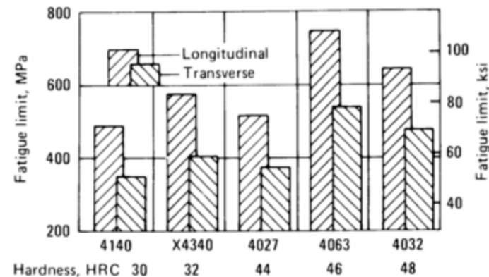
Fig. 12 Effect of specimen orientation on fatigue limit. Orientations are relative to the fiber axis resulting from hot working on the fatigue limit of low-alloy steels.
