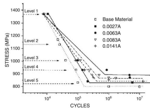
Fig. 14 S-N curves of AISI 4340 steel shot peened are compared with the base metal.
