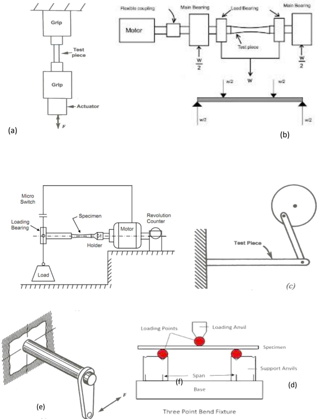
Fig. 2 Different types fatigue testing arrangements (a) axial loading, (b) rotating-bending, (c) rotating cantilever bending, (d) constant deflection amplitude cantilever bending, (e) combined in-phase torsion and bending and (f) three point flexural fatigue testing system.
