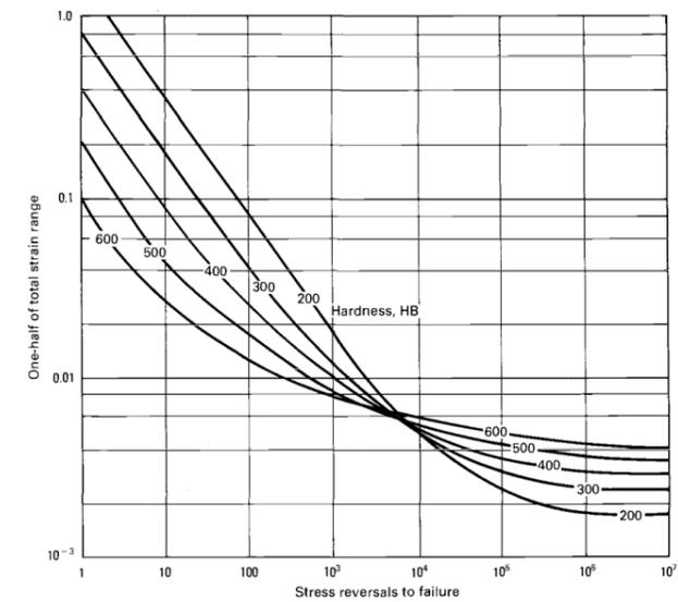
Fig. 7 Effect of hardness level on plot of total strain versus fatigue life.
