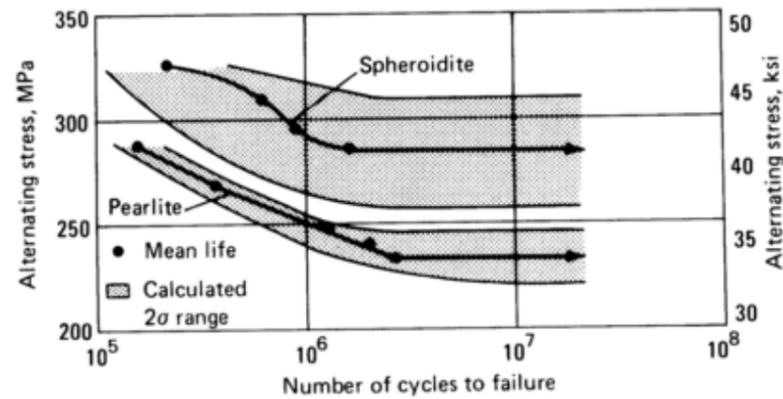
Fig. 5 Effect of microstructure on fatigue behavior of carbon steel (0.78% C, 0.27% Mn, 0.22% Si, 0.016% S, and 0.011% P).
