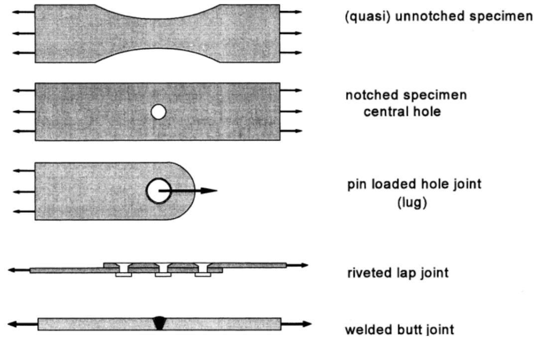
Fig. 1 Different types of simple fatigue specimens.
