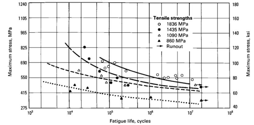
Fig. 6 Room temperature S-N curves for AISI 4340 alloy steel with various ultimate tensile strengths and with R = -1.0.
