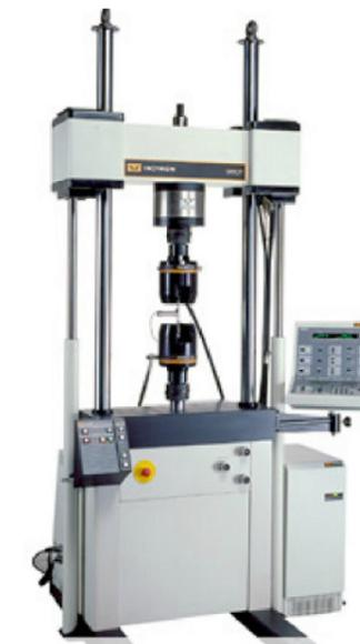
Figure 16 Servohydraulic testing frame for axial loading
