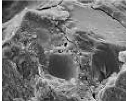
Fig. 1: Micro-crack in concrete (After Stark, 2006)
